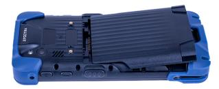
2. Press in and hold the two plastic clips at the end of the battery, then push the battery forward and down into the battery compartment.
