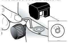
Check the circular bubble vial by rotating the telescope by 180°. If required, repeat the procedure or refer to an authorized SitePro after-sales service.
