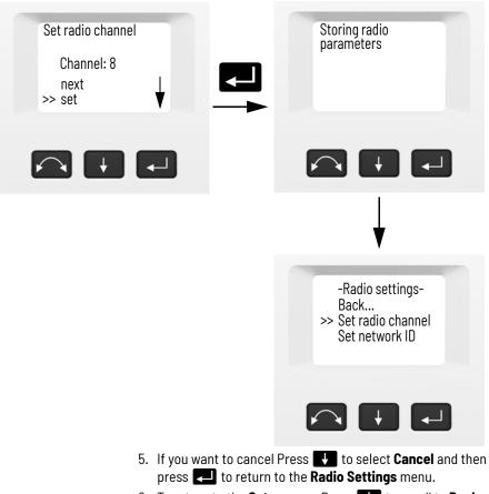
6. To return to the **Setup** menu Press V to scroll to **Back** and then press V.
