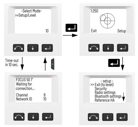
**Note -** If no selection is made within 10 seconds the instrument will go to suspend mode. To return to the select mode menu press the trigger key.
