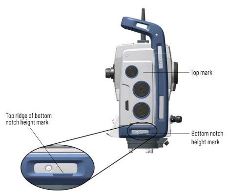
When there is a Spectra Geospatial data collector connected running a field application software, the software has additional functions that reduce the bottom notch height mark measurement to the required vertical instrument height to the trunnion axis.
