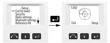
**Note** - If the instrument is left idle for more than 300 seconds (5 minutes) during any of the above routines, then the instrument goes to suspend mode.
