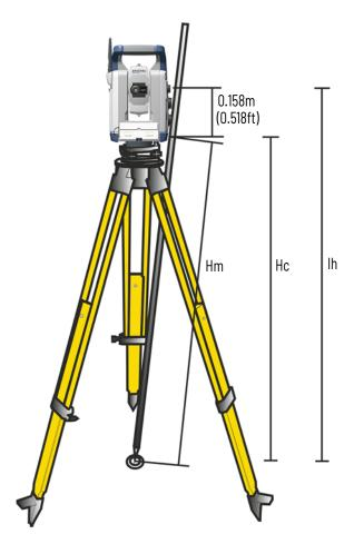
The measured distance (Hm) is corrected for the slope of the measurement to obtain a vertical measurement to the bottom notch height mark (Hc). The constant from the bottom notch height mark to the true height mark (0.158 m/0.518 ft.) is added to the Hc to obtain the vertical instrument height from the ground mark to the trunnion axis (Ih). For more information, refer to the field software documentation.
