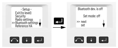
2. To change the Bluetooth device setting press 🛃 to select **Next** and then press 💶 to select **on** or **off**.
