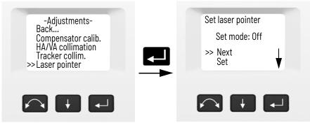
2. To change the laser pointer setting, press 🚺 to select **Next** and then press 💶 to select **On** or **Off.**
