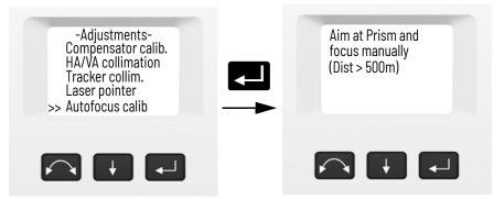
3. Aim and manually focus at a target at a distance of at least 500 meters, then press
