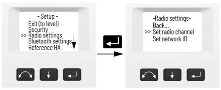
3. To change the radio channel number press 🛃 to select **Next** and then press 💶 to change the channel number in the display.
