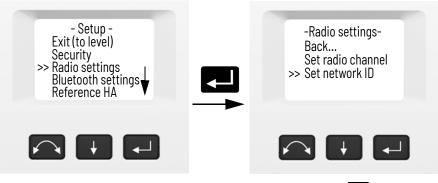
3. To change the network ID number press 🛃 to select **Next** and then press **L** to change the channel number in the display.
