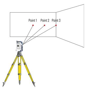
With offset measurements, you can accurately measure difficult locations with DR instruments, and eliminate beam divergence errors. For more information, refer to the field application software documentation.
