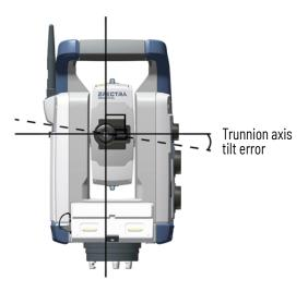
In the instrument, perform a pre-measurement trunnion axis tilt test to determine the trunnion axis tilt error. Angular measurements are observed in both instrument faces, the trunnion axis tilt error is calculated, and the respective correction value is stored in the instrument. The trunnion axis tilt correction value is then applied to a correction to the horizontal angle value and an automatic repointing of the telescope using SurePoint technology.
