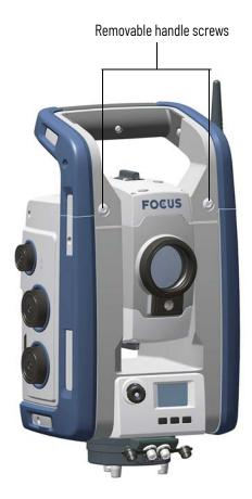
2. Slide the handle horizontally away from the front of the instrument.
