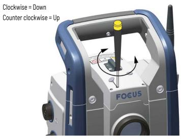
3. To correct the horizontal position of the laser spot, insert the Allen key into the horizontal adjustment port and turn it.
