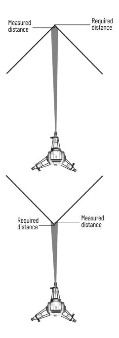
Although the problem is reduced with a beam that uses a smaller measuring area, the error can not be completely eliminated. The most accurate solution to measure to tight corners and eliminates errors caused by beam divergence, is to use an offset measurement method such as that used in the field application software:
