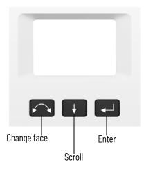
When a secondary function is available on a button, an icon appears at the bottom of the display. To access the secondary function, press and hold the appropriate key.
