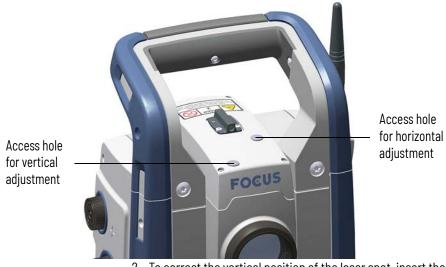
2. To correct the vertical position of the laser spot, insert the Allen key into the access hole for the vertical adjustment screw and turn it.
