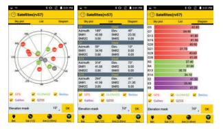
To change the value of elevation mask shown at the bottom of the screen, just touch the current value and type in the desired value. Then touch **OK** to validate the new value. NOTE 1: All GNSS constellations are tracked by default but you may deselect one (or more), if desirable, by clearing the corresponding check box shown on this screen.
