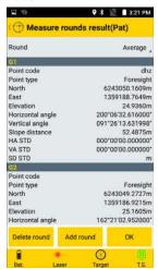
Set **Round** to either view the individual measurements for each point and each round (select 1 or 2 or 3, etc.), or for
