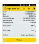
Note that the point name is automatically incremented at the end of the measurements so you don't need to type a new name for the next point.
