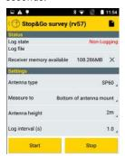
Touch the yellow Start button. Survey Mobile starts logging GNSS raw data for your current location. A new screen is displayed showing the data logging status ("Logging"), the name of the opened raw data file and the amount of memory available on the receiver.
