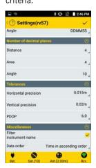
Filter instrument name: When requested to scan for Bluetooth devices, Survey Mobile will either list the names of all the detected Bluetooth devices (case where the Filter instrument name option is disabled), or
