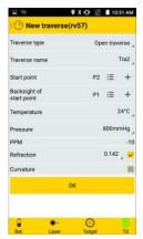
Touch **OK** to save the traverse. After saving the traverse, Survey Mobile returns to the **Tools** menu.
